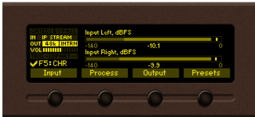
Left and Right Audio Input Levels (dBFS), represented as bar graphs.
