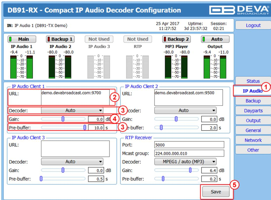
The screenshot displays the configuration page for the DB91-RX decoder. At the top, it shows system information like 'IP Audio 1 (DB91-TX Demo)', date, and uptime. Below are several audio level meters for Main, Backup 1, Not Used, Not Used, Backup 2, and Auto. The main configuration area is divided into sections for IP Audio Client 1, IP Audio Client 2, IP Audio Client 3, and an RTP Receiver. Red annotations highlight the following elements:
