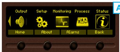
Using the [RIGHT] navigational button find the **Status** section located at the end of the Menu (A).
