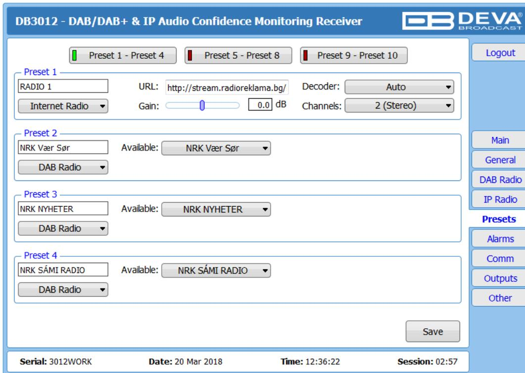
The DB3012 allows 10 user presets to be set and saved in the device's memory. The procedure of adding a new preset is quite simplified.
