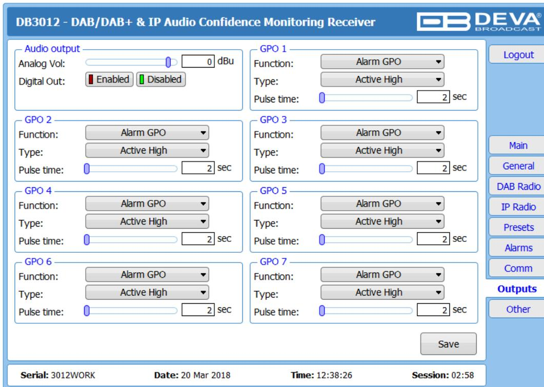
The general purpose outputs settings are applied through this page. The *Audio output* section allows *Audio Vol* for the analog output to be set, and the *Digital Out* to be [Enabled] or [Disabled].
