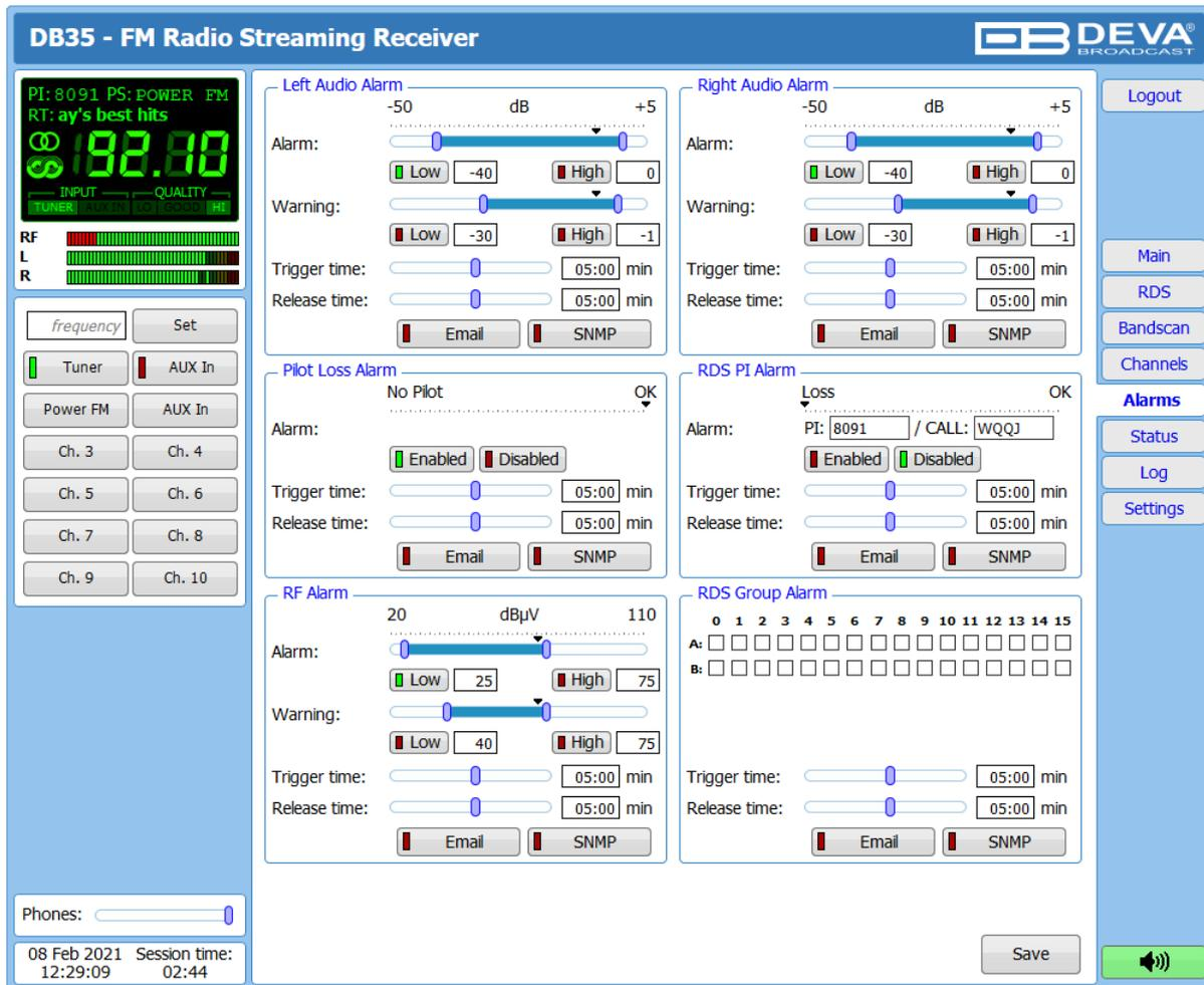
DB35 has a set of the six parameters that can be monitored: Left and Right audio levels, RF Level, Pilot Presence, RDS PI and RDS Groups. Trigger and alarm release times can be set for each alarm. The notification means (Email and SNMP) is set for each parameter individually. To enable the notification, press on the relevant button so that it could be illuminated in green.
