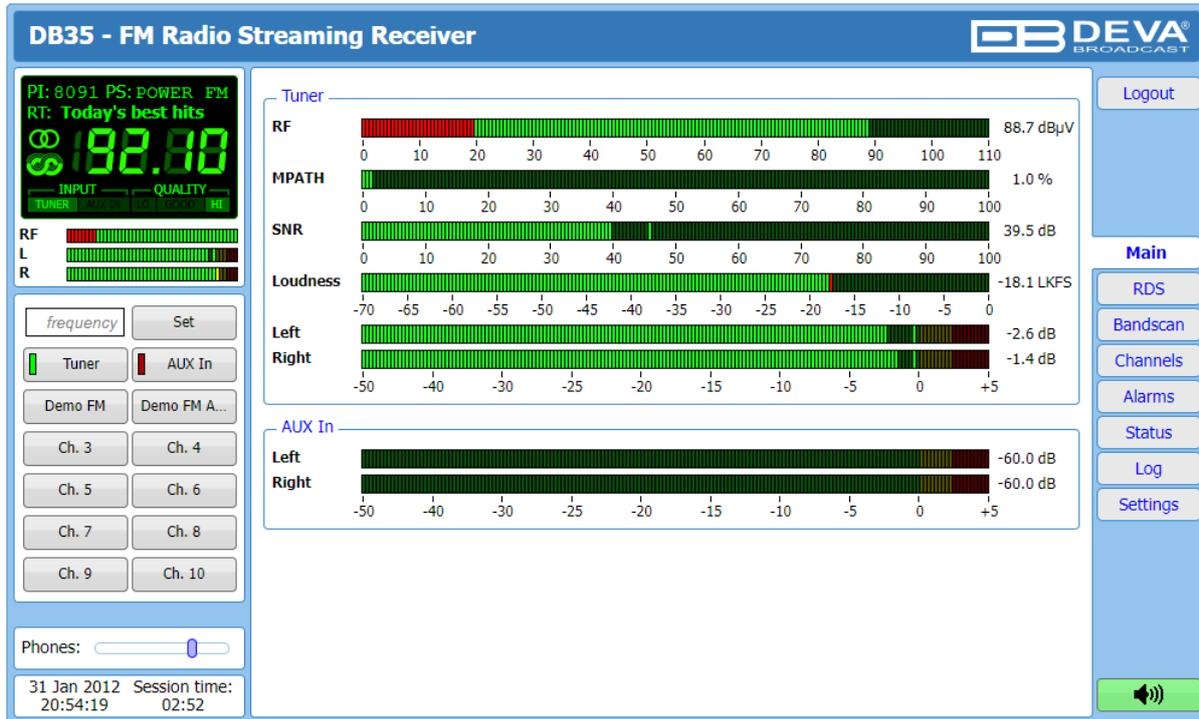
The Main Screen of the WEB Interface shows all the mandatory parameters represented as LED readings. You can easily select the preferred audio frequency by using the selection buttons, placed on the left part of the screen. All station presets are defined by the user.
