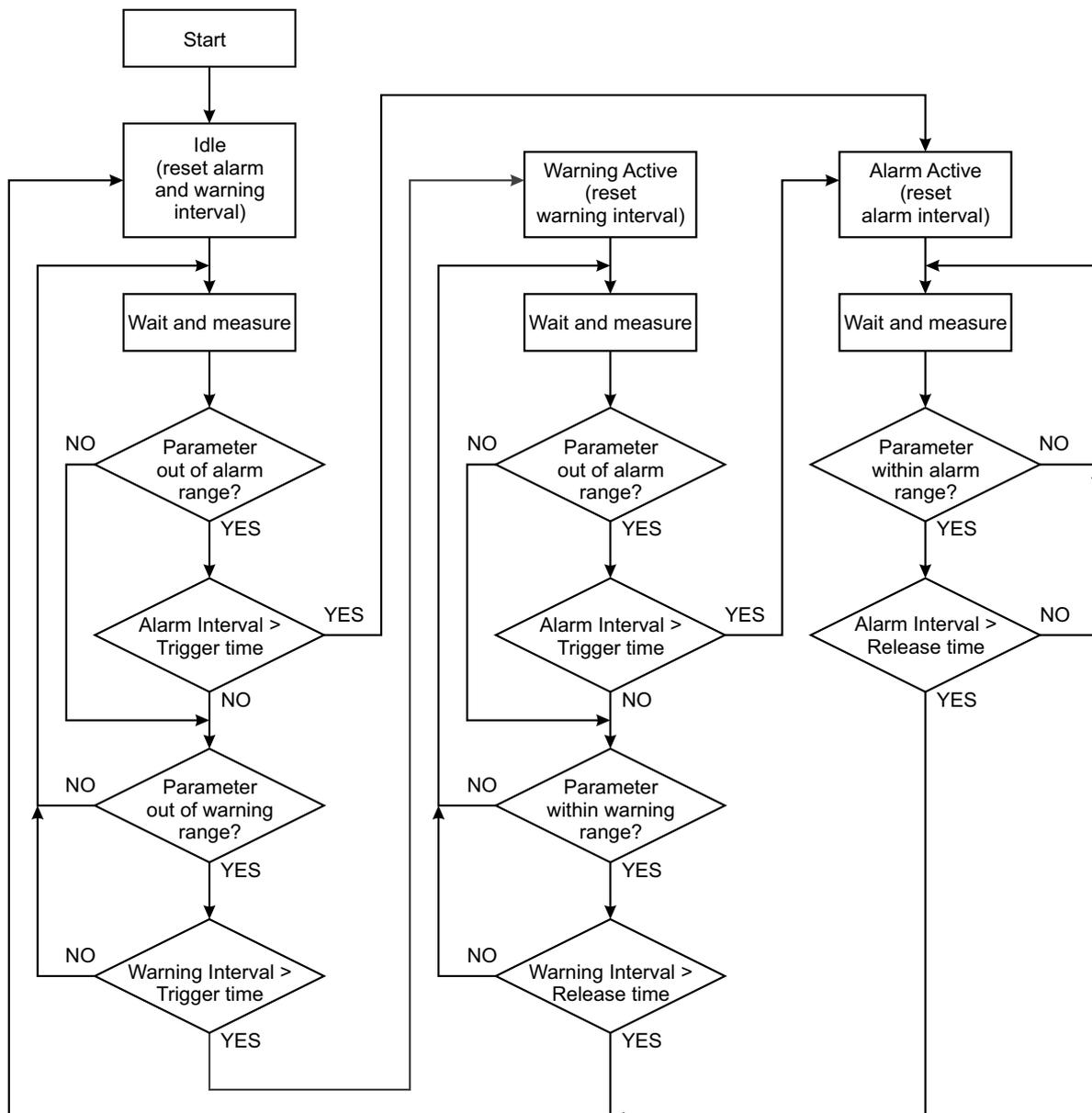
*Block Diagram of Alarm Automata*
