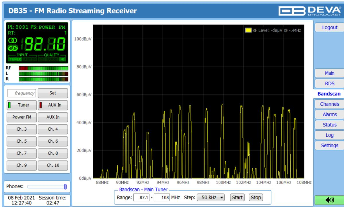
This Screen evaluates FM broadcast band congestion by sweeping the tuner across the FM band, logging every carrier and generating a spectrum display of carrier level vs. frequency.
