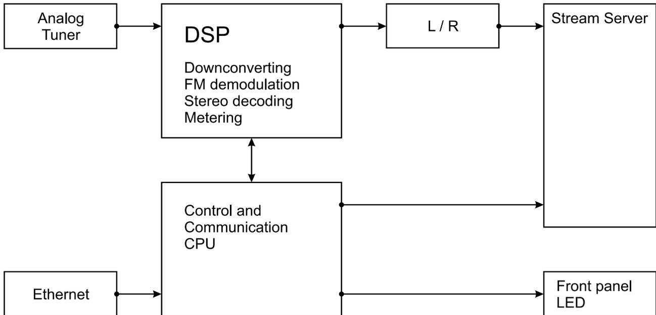
Because of the all-digital, minimalist-discrete-component nature of device circuitry, we have not provided schematic diagrams of the DB35 in this Manual. Please, note that:
