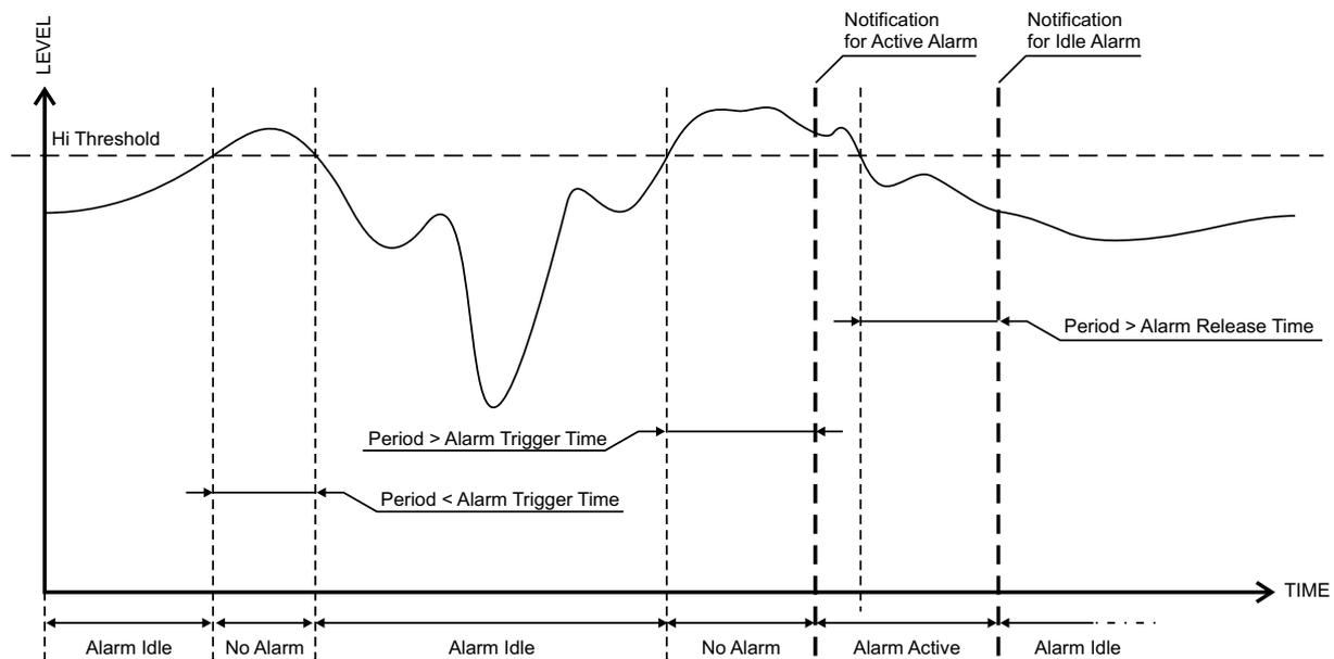
If the RDS Group has not been received within the Alarm Trigger Time, the state would be changed into Active. If the Active state and the Release Time have elapsed and the RDS Group is received, the state is changed to Idle. Should the RDS Group is received before the Release Time is elapsed, the state would remain Active.
