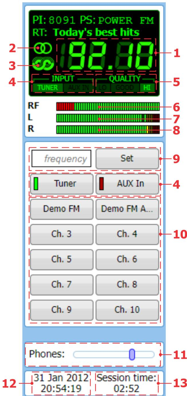
1. Frequency indicator showing currently tuned frequency;
