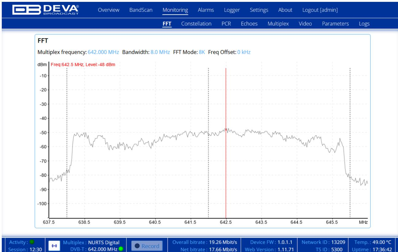
The Discrete Fourier Transform is a simple but fairly time-consuming algorithm. To obtain the precise result of the Fourier Transform, a time-domain signal would have to be observed for an infinitely long period of time. In the case of the Discrete Fourier Transform, however, a signal segment is only observed for a finite period of time and transformed. The result of the DFT or FFT, respectively, will thus always differ from that of the Fourier Transform.
