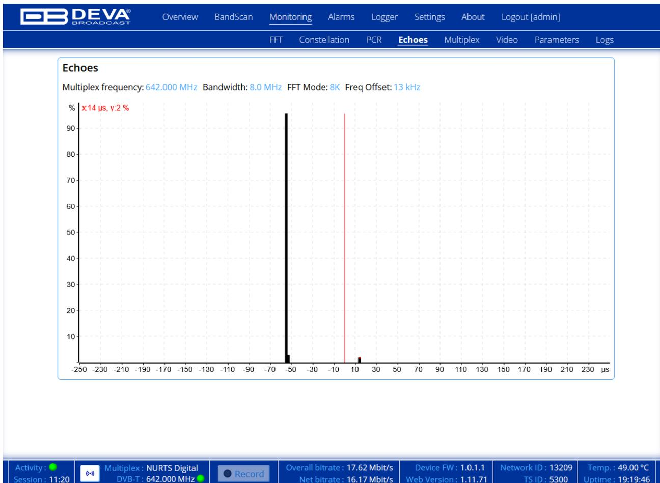
This view displays the instantaneous Channel Impulse Response detected by the receiver. User can check the power level and delay of other echoes from main echo by dragging the red line pointer over the echo. Values are displayed in the upper left corner of the graph (in red color).
