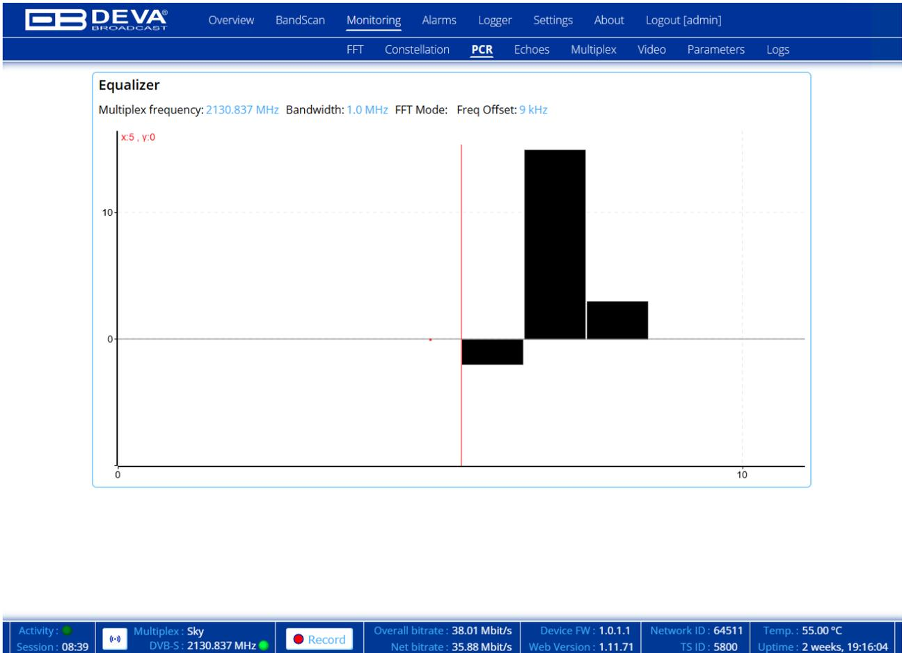
The digital channel equalizer serves to correct transmission errors. The channel equalizer block also includes a matched filter which performs roll-off filtering.
