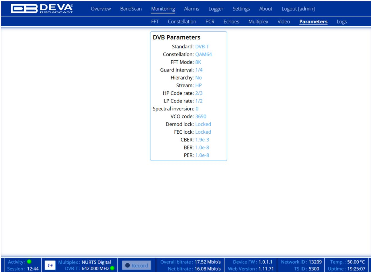
The screenshot shows the DEVA Broadcast web interface. The top navigation bar includes: Overview, BandScan, **Monitoring**, Alarms, Logger, Settings, About, Logout [admin]. Below this, a secondary navigation bar includes: FFT, Constellation, PCR, Echoes, Multiplex, Video, **Parameters**, Logs. The main content area displays the following DVB Parameters:
