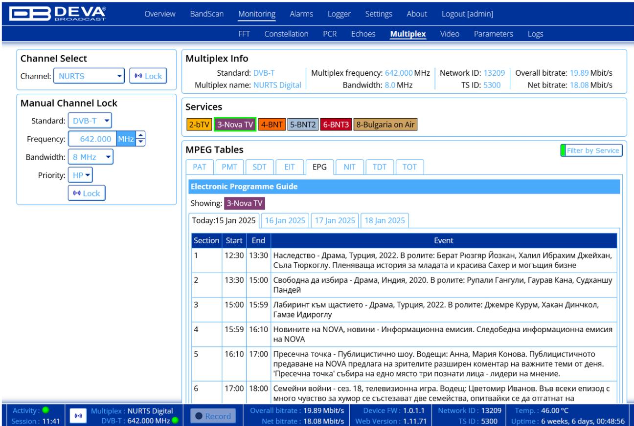
The screenshot shows the DEVA Broadcast Monitoring interface. The top navigation bar includes: Overview, BandScan, Monitoring (selected), Alarms, Logger, Settings, About, Logout [admin]. Below this is a secondary navigation bar with: FFT, Constellation, PCR, Echoes, Multiplex (selected), Video, Parameters, Logs.
