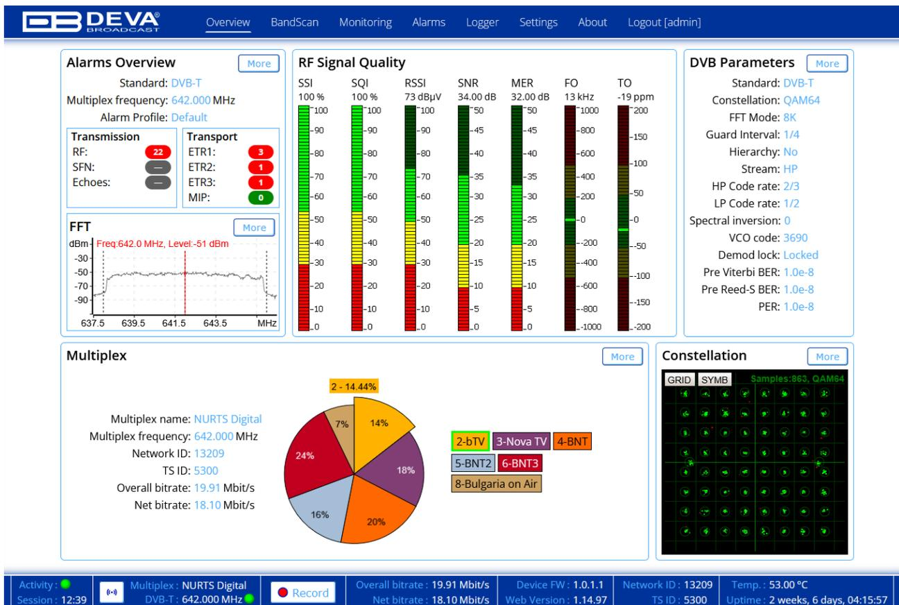
The main window is functionally divided into five main panels – **Alarms Overview**, **RF Signal Quality**, **DVB Parameters**, **Multiplex** and **Constellation**. This allows you to have a quick view of all the mandatory parameters. A click on the [More] button (placed in the top right corner of each section) will lead you to the WEB page of the relevant parameter/data.
