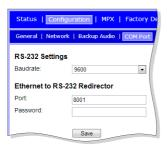
DB9000-STC acts as Ethernet to an RS-232 redirector. You can connect any RS-232 compatible equipment to DB9000-STC and to communicate with it over the Internet. A special software (Virtual COM Port to Ethernet Tool) need to be installed on your PC in order for the COM Port configuration to take place. Enter a Baudrate and configure the external equipment to the same baud rate, specify Port and Password next.
