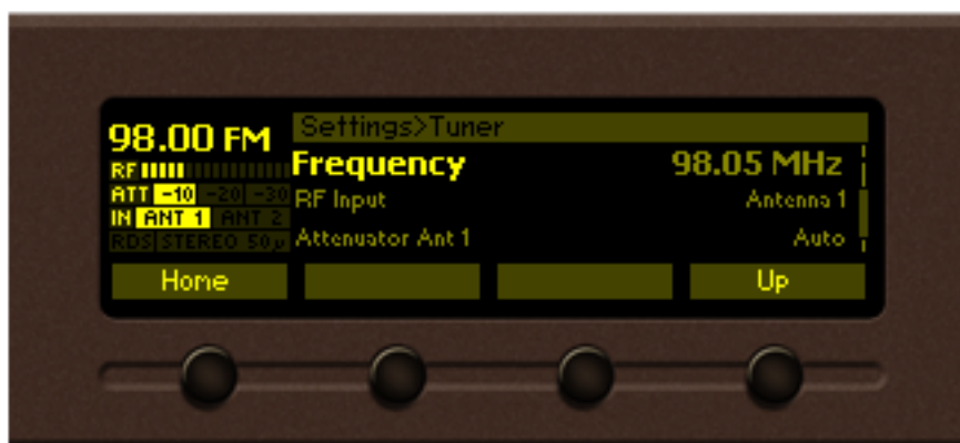
“Frequency” parameter from “Tuner” branch
