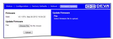
To update the device firmware, please select the new firmware file. Press the Upload button. A dialog window will appear. Confirm firmware update and wait for the process to complete.
